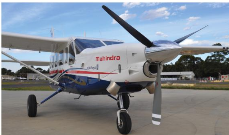
The Rolls Royce M250 powered Airvan 10 has a larger market than its piston-powered sibling.
